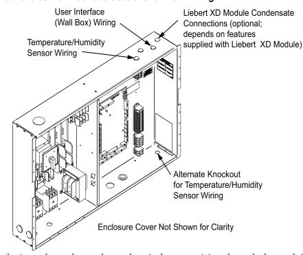
Figure 11 Electrical enclosure knockout locations for field wiring
